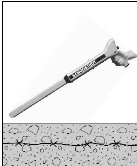
Figure 17. Tracing Barbed Wire
